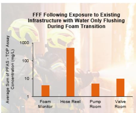
With water only flushes on the fire suppression system, PFAS buildup rebounded at up to 1.6 g/L in fluorine-free firefighting foams
