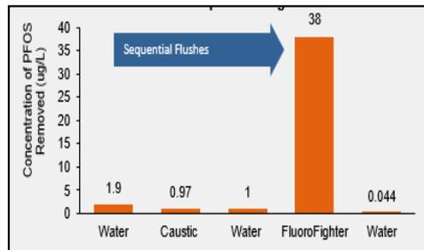
*FluoroFighter™ was most effective at removing PFAS from the AFFF impacted system.*
