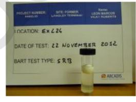
BART<sup>™</sup> Test Type: Sulphate Reducing Bacteria
