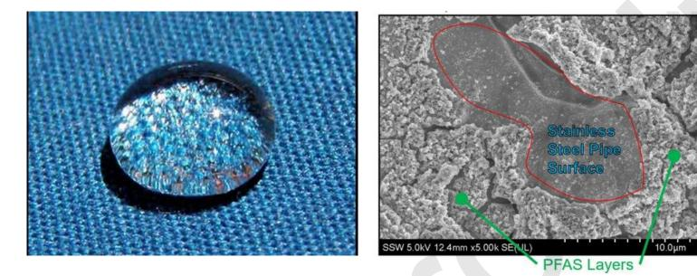
structures will build up in layers on the interior surfaces
