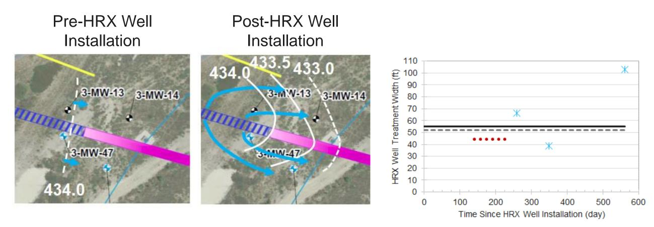
**Figure 8. Left:** Change in local hydraulic gradient before (left) and after (right) HRX Well installation. Right: Capture zone width calculated by Darcy's Law (solid black line), the numerical flow model (dashed grey line), HRX Well tracer test (dotted red line), and PVP tests (blue stars).
