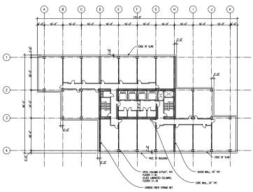
Mass timber floor plan 16'-0" grid
